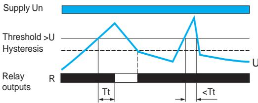
If the controlled voltage exceeds the threshold setting for a time greater than that set on the front panel (0.1...30 s), the output relay opens and the R LED goes off. During the time delay, this LED flashes.
