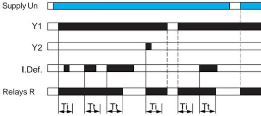
This mode is designed to control a pump via an external signal. The relay output is closed when the signal is present at Y1 (contact closed). Y2 can be used to reset the relay after a current fault.
