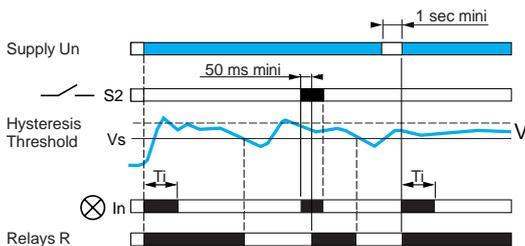
When relay RM35S has been configured in “memory” mode, if underspeed is detected, the output relay stays in the “open” state, irrespective of any further changes in the process speed.
