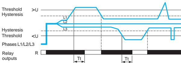
**Note:**  $T_t$ : time delay after crossing of the threshold (adjustable on the front panel)
