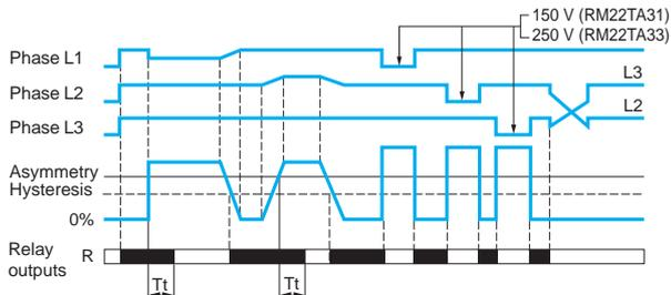
The relay monitors its own supply voltage  $U_n$ :
