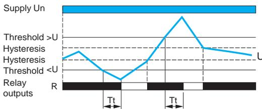
These relays operate in window mode where they check that the controlled voltage stays between a minimum and a maximum threshold.
