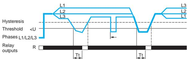
**Note:**  $T_t$ : time delay after crossing of the threshold
