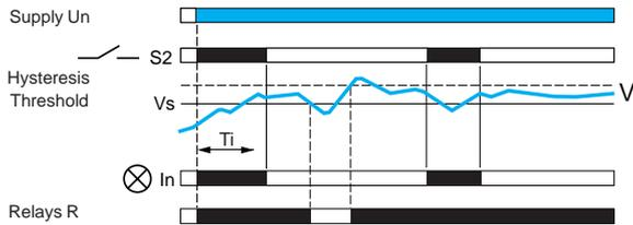
On energization, to allow the process being monitored to reach its nominal operating speed, relay RM35S is inhibited for a time delay adjustable from 0.6...60 s. This time delay can be adjusted (shortened or lengthened) during inhibition.
