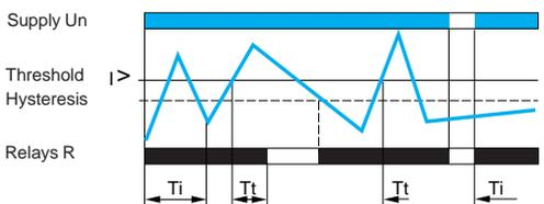
If the current controlled exceeds the threshold setting for a time greater than that set on the front panel (0.3...30 s), the output relay opens and the LED goes off. As soon as the current drops below the value of the threshold setting minus the hysteresis, the relay instantly closes.
