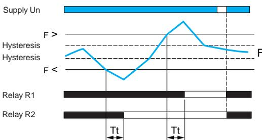
If "Memory" mode is selected, the relay opens after the time delay and stays in that position when crossing of the threshold is detected. The power needs to be switched off to reset the product.
