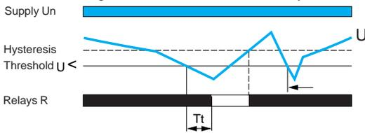
If the voltage controlled falls below the threshold setting for a time greater than that set on the front panel (0.3...30 s), the output relay opens and the **R** LED goes off. During the time delay, this LED flashes. As soon as the voltage rises above the value of the threshold setting plus the hysteresis, the relay instantly closes.
