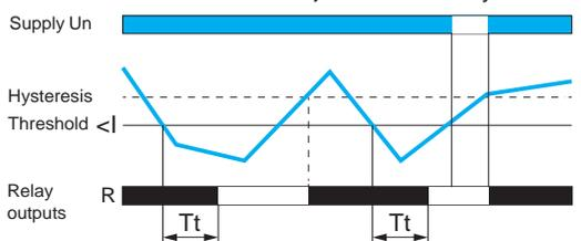
If the controlled current falls below the threshold setting for a time greater than that set on the front panel (0.1...30 s), the output relay opens and the R LED goes off. During the time delay, this LED flashes.
