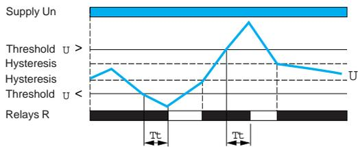
These relays operate in window mode where they check that the controlled voltage stays between a minimum threshold and a maximum threshold.
