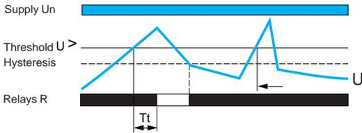
If the voltage controlled exceeds the threshold setting for a time greater than that set on the front panel (0.3...30 s), the output relay opens and the **R** LED goes off. During the time delay, this LED flashes. As soon as the voltage drops below the value of the threshold setting, minus the hysteresis, the relay instantly closes.
