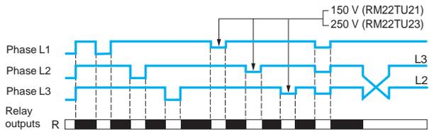
The relay monitors its own supply voltage  $U_n$ :
