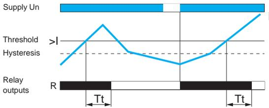
If "Memory" mode is selected, the relay opens when threshold crossing is detected and then stays in that position. The power has to be switched off to reset the product.
