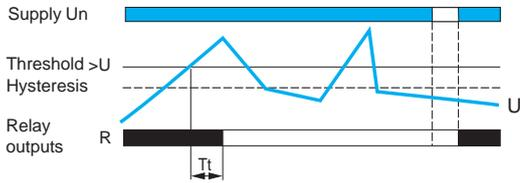
If "Memory" mode is selected, the relay opens when crossing of the threshold is detected and then stays in that position. The power has to be switched off to reset the product.
