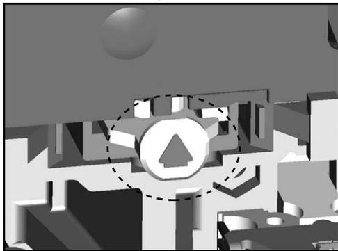
Place a projection matching with its groove, or position two triangle labels to be on the same line.
