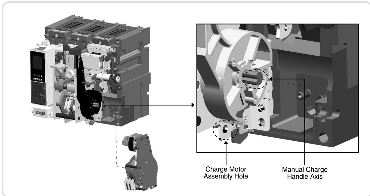
3) Tighten with M6 bolt after fitting the bottom of charge motor into the bottom of mechanism.
