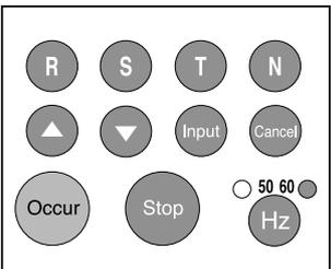
**R S T N** R, S, T, N phase signal input (Size/Phase)
