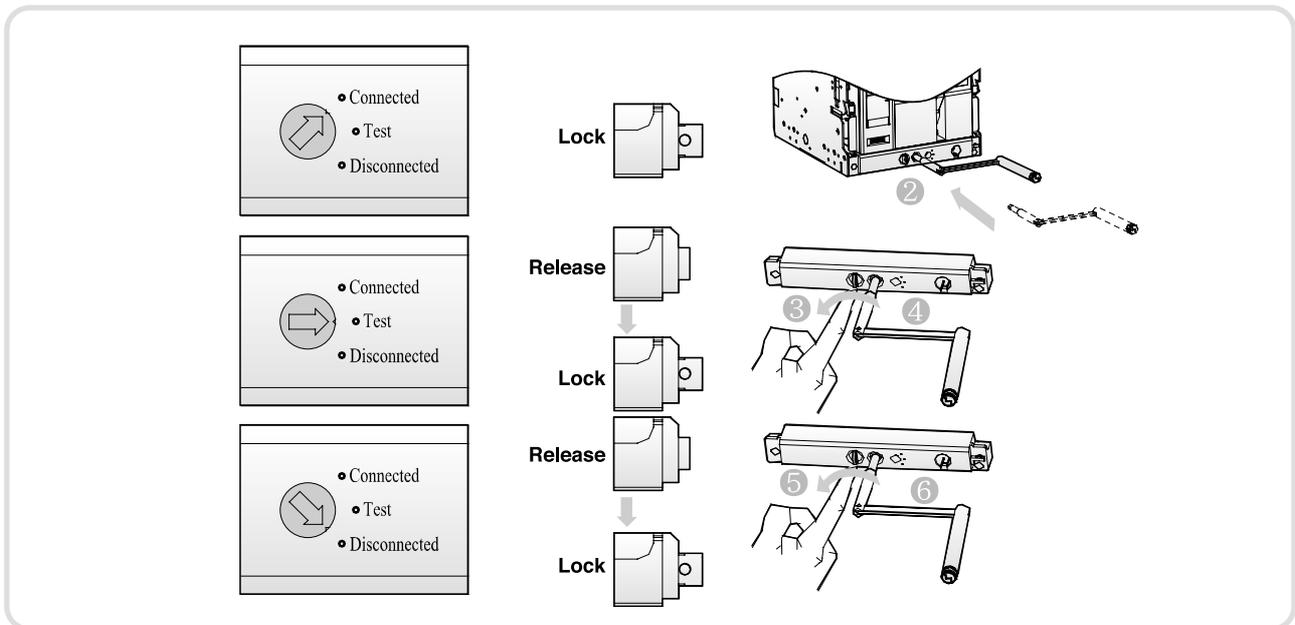
5. The circuit breaker indicated with 'DISCONNECTED' can be separated safely from the cradle by removing a draw in/out handle and releasing right and left locks.
