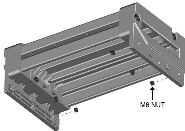
2) Put 6pcs of M6 Bolt into holes of Arc cover and both Side plates and then tighten them.
