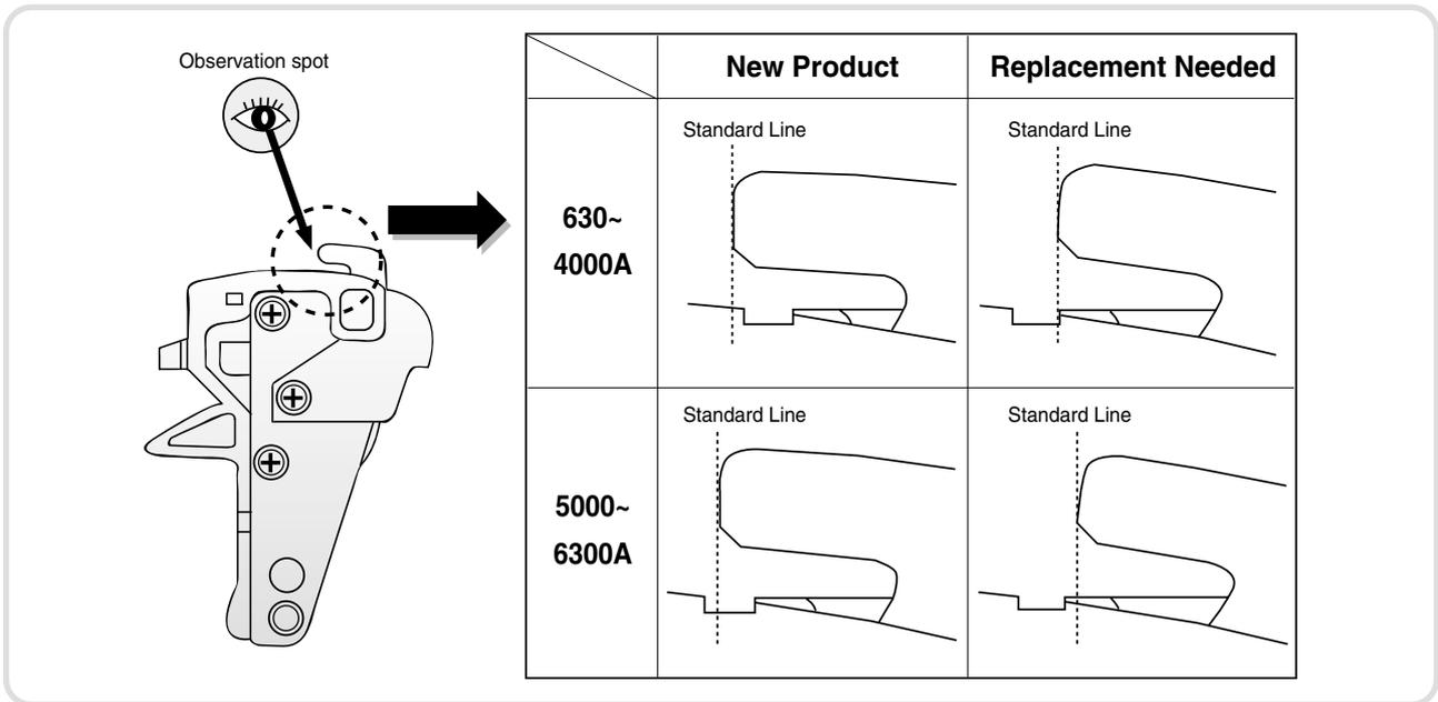
Fig 8. The standard figure for contact replacement
