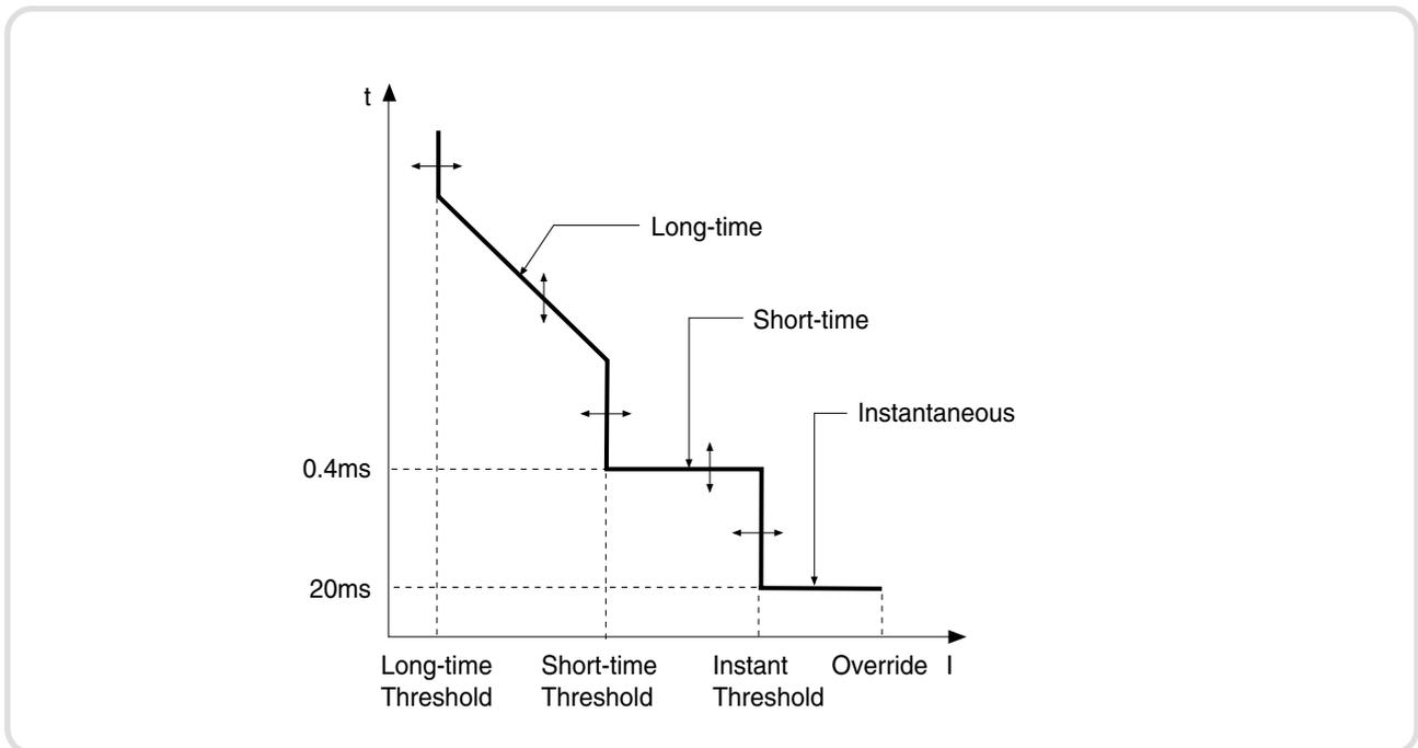
Picture1. Low Voltage Circuit Breaker's Characteristic Curve
